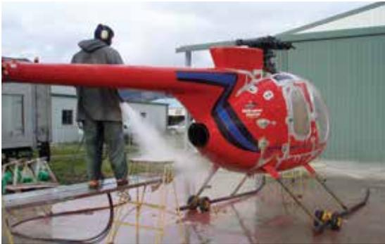
Over the last 8 years, Aquamax has successfully completed surface preparation on 135 aircraft throughout New Zealand. These jobs have involved coatings removal as well as filiform corrosion excavation. Aquamax operators have more than 4350 hours' experience in the removal of surface coatings from aircraft.
