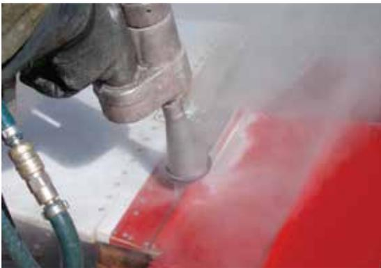
Each of our mobile units is fully self-sufficient, holding 1800 litres of water, which enables 8 hours' blasting time. The pump units use only 3.2 litres of water per minute.
