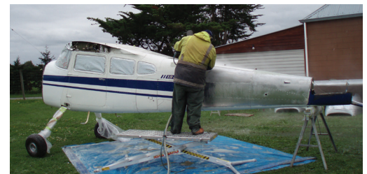
Low flow-rate water jetting
