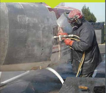
Aquamax has been active in the general aviation (GA) sector for over 12 years. We are known for our unique aircraft paint stripping process, an attractive alternative to using chemical strippers and abrasive methods. We have developed this process in conjunction with industry ensuring an appropriate level of documentation and process checks.
